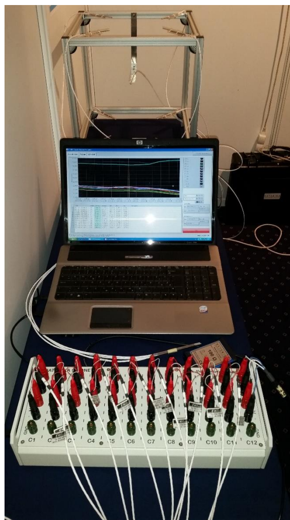
UT-ONE S12A thermometer readout with 12 Elpro Pt-100 probes demonstrating the validation of climatic chambers
