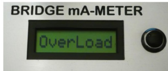
Indication of OverLoad condition
